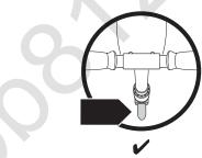
**2** With the front wheel pointed straight ahead and the handlebars square to the front wheel and the Razor logo facing the front, tighten the clamp as shown. Tighten securely.
