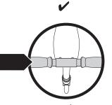
**WARNING:** Failure to properly engage the spring-loaded buttons may cause the handlebars to dislodge while riding and may cause rider to lose control and fall. When correctly engaged, the handlebars will not rotate nor move sideways, and the spring-loaded buttons will be clearly visible in the holes on the T-bar.
