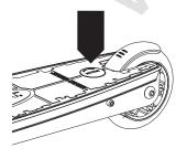
**1** To activate the batteries, locate the battery compartment on the top of the deck and remove the plastic tab from under the battery cover.
