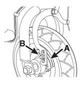
**3** Inspect the brake pads (A) for proper alignment against the wheel or excess wear. To realign brake pads, loosen the fixing nut (B) and adjust the pad to contact the rim. Retighten and test. Readjust as needed.
