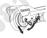
**3** To loosen the chain, push the tensioner down to create some slack in the chain.
