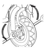
2 Using two 17mm wrenches, loosen the locknuts by turning the wrenches counter clockwise. Remove wheel and install replacement wheel.
