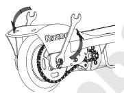
**2** Using two 13mm wrenches, loosen the locknuts by turning the wrenches counter clockwise.
