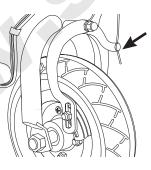
**2** If brake is too tight or has too much slack, use a 10mm open wrench to loosen the brake cable and adjust accordingly.
